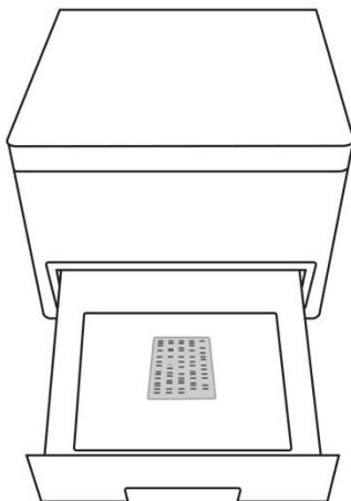
3. Place the UV protection shield on the drawer. The shield placement is secured by the magnet.
